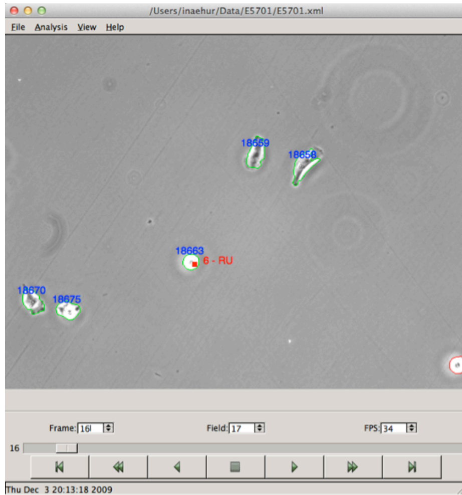
Figure 1. casViewer. Main window of casViewer shows segmented cell with id, event number, and designation. Cells with green border represent an actual cell; objects with a red border are partial cells or alter artifacts which can then be ignored in subsequent analysis.
